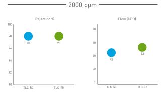
Product Tested at 65 psi; 77°F; 20% recovery; 2000 ppm NaCl/RO
