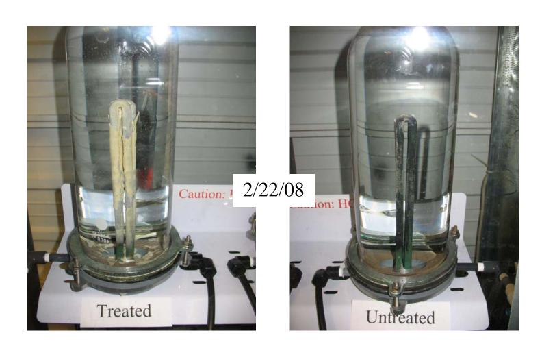
Here is a close up of the heating element that was feed untreated water for two weeks then treated water for three weeks. Notice the scale flaking off of the element. Also notice the flakes of scale on the bottom of the chamber. This picture was taken on 2/22/08.
