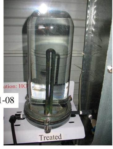
The tubing was changed on 2/01/08 and we began sending treated water to the scaled up chamber and untreated water to the clean chamber. The pictures below were taken three days after changing the tubing.
