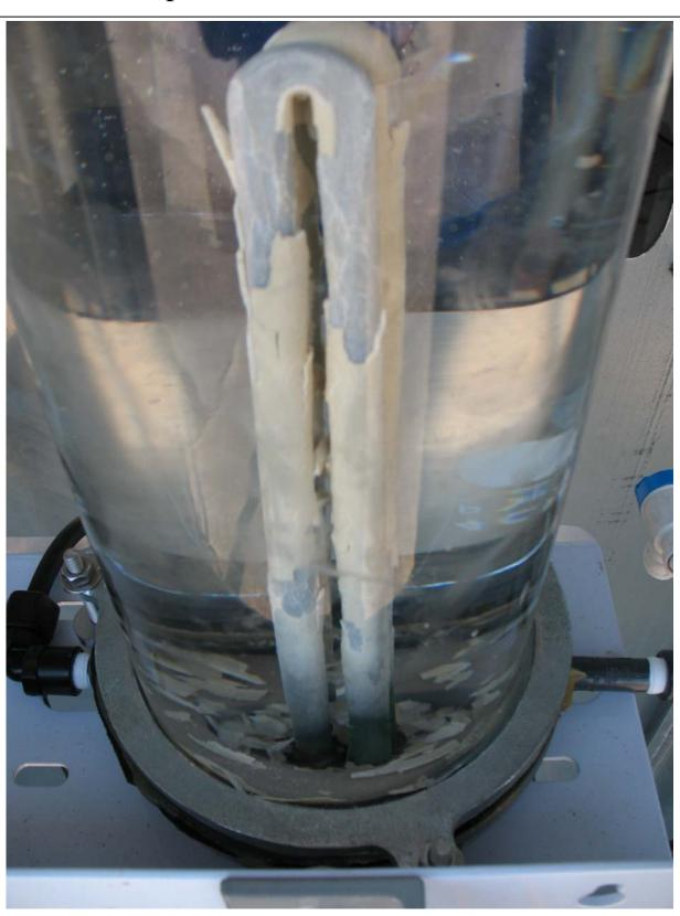
Here is a close up of the heating element that was feed treated water for two weeks then untreated water for three weeks. Notice how little scale has accumulated. This picture was taken on 2/22/08.
