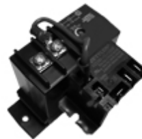
Current Sensor Switch - Part# M 120150 Operates 110 volt chlorinators with adjustable current sensitivity (used exclusively with 110 volt chlorinators during VFD applications which require “Clean” 60 Hz
