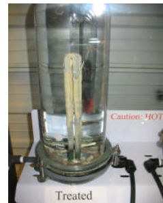
De-Scaling (After sending treated water to scaled-up heating element.)
