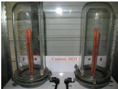
Side-By-Side Test Stand (To test untreated and treated water.)
