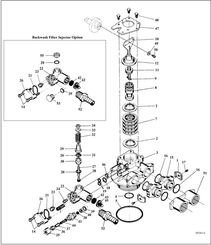
Figure 13: Model 5600 and 5600 Econominder Control Valve Drive Assembly
