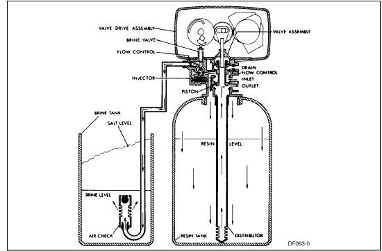
Figure 11: Brine Tank Fill Position
