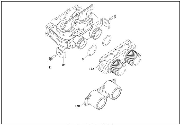
Figure 15: Bypass Valve Assembly, Plastic
