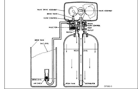
Figure 10: Settling Rinse Position
