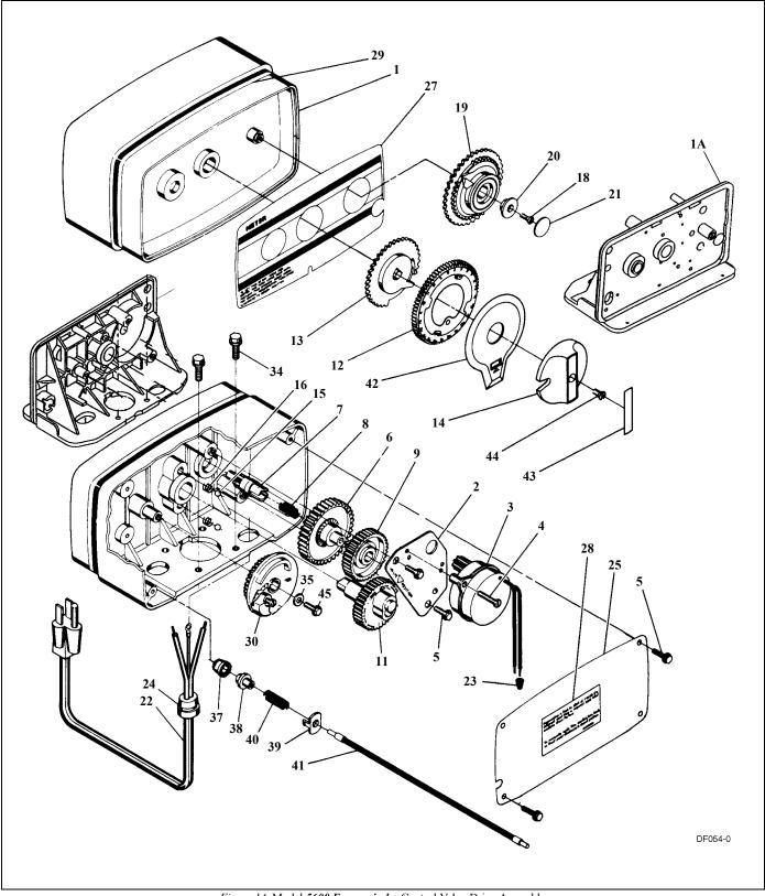
Figure 14: Model 5600 Econominder Control Valve Drive Assembly
