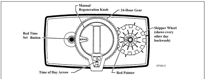
Figure 2: Model 5600 Backwash Filter Control
