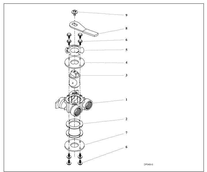
Figure 16: Bypass Valve Assembly, Brass
