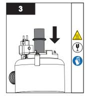
Place O-ring on the sleeve as shown. Insert the sleeve into the chamber as shown in step 4.
