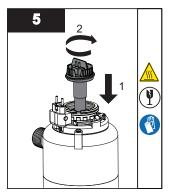
Insert new lamp into the quartz sleeve and thread into sleeve bolt until hard stop.
