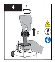
• Hold sleeve bolt with one hand and turn lamp counterclockwise and pull the lamp outside the chamber in upward direction.
