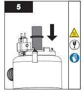
• Place O-ring on the sleeve as shown. Insert the sleeve into the chamber as shown in step 6.
