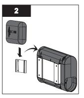
Slide controller onto mounting bracket.
