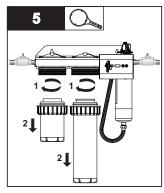
• Remove the sump housings using sump wrench.
