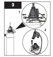
• Remove the lamp connector by pulling the tabs out and then upwards.
