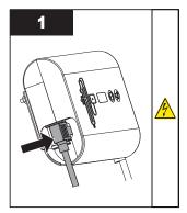
Ensure the controller is plugged in for entire cleaning process.
