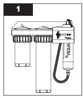
Install the UV system on the wall using lag bolts (not supplied). Mounting holes are located in the metal bracket.
