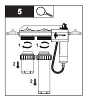
Remove both the housing(s) using sump wrench.
