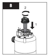
• Insert lamp into the quartz sleeve and thread into sleeve bolt until hard stop.
