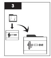
• Insert the reference card between controller and mounting bracket.
