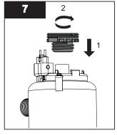
Place sleeve bolt onto the quartz sleeve, carefully push down and hand tighten onto chamber.
