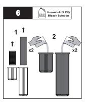
Remove cartridges and pour 2 cups of household bleach solution into the sump housings.
